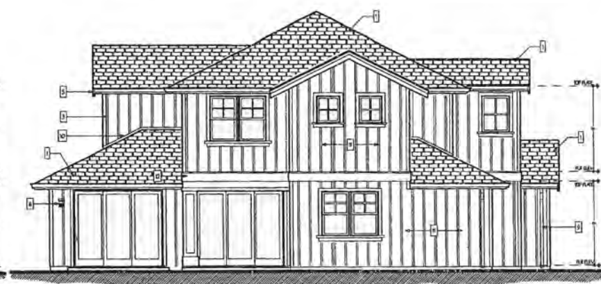
4 Rear Exterior Elevation [ South ] Scale: 1/4" = 1'-0"
